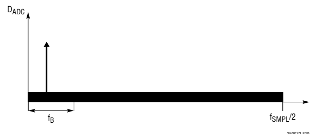
Figure 20. Frequency Spectrum of SAR ADC Core Output
