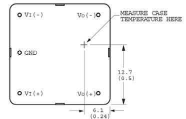
Note: Top view, pin locations are for reference only. Measurements are shown in millimeters and (inches). 1-0146
