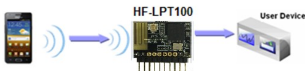
Figure 24. Wireless Control Application
