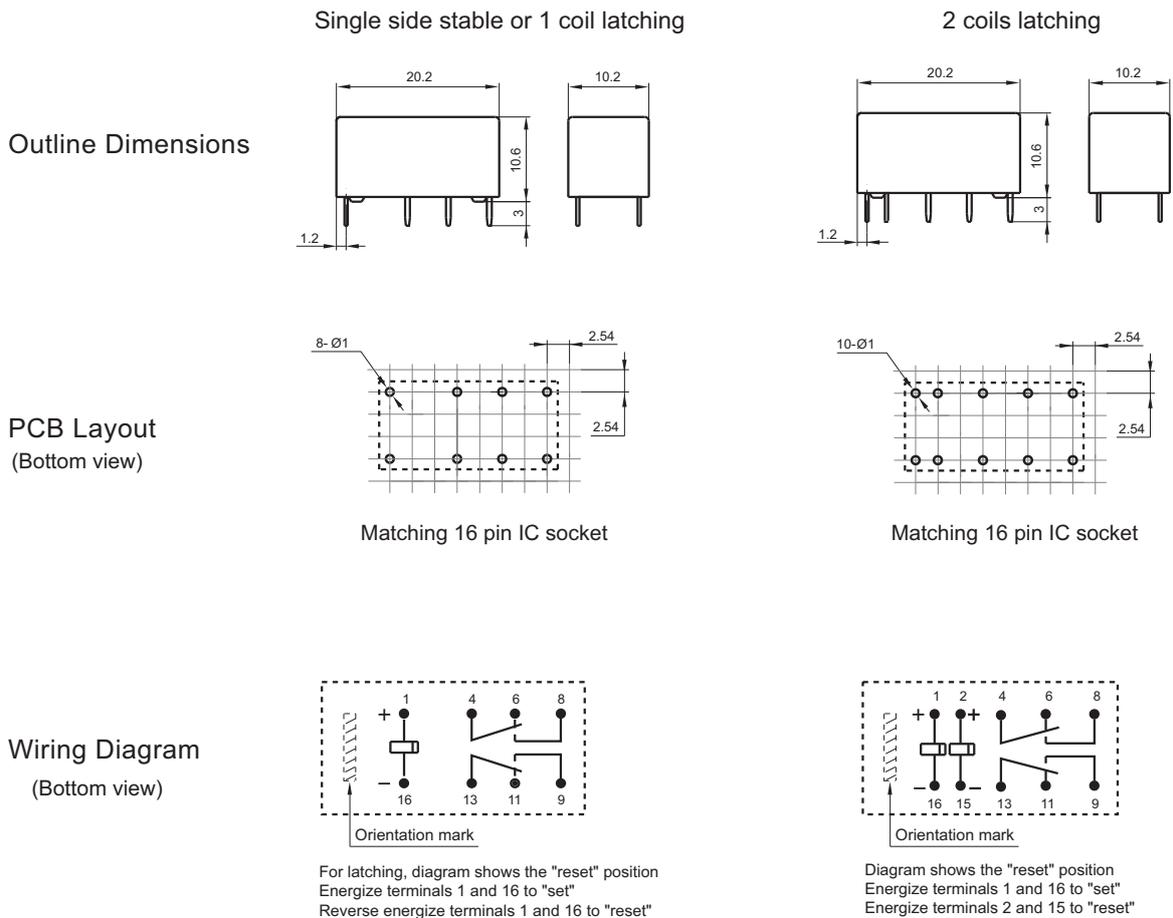
Remark: 1) In case of no tolerance shown in outline dimension: outline dimension  $\leq 1$ mm, tolerance should be  $\pm 0.2$ mm; outline dimension  $> 1$ mm and  $\leq 5$ mm, tolerance should be  $\pm 0.3$ mm; outline dimension  $> 5$ mm, tolerance should be  $\pm 0.4$ mm.
