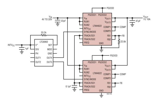
Figure 28. 4 Phase, 1V Output at 10A Design with LTC6902
