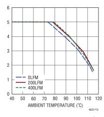
Figure 15. 5V to 1.5V Derating Curve, No Heat Sink
