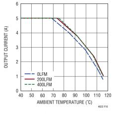
Figure 16. 12V to 1.5V Derating Curve, No Heat Sink
