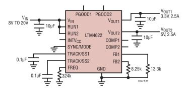
Figure 26.  $8V_{\mbox{\scriptsize IN}}$  to  $20V_{\mbox{\scriptsize IN}},\,3.3V$  and 5V Output at 2.5A with 2MHz Switching Frequency
