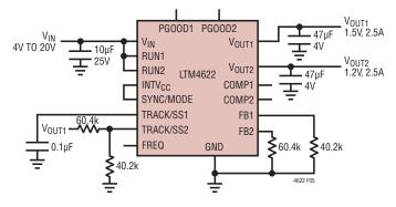
Figure 5. Example Schematic of Ratiometric Output Voltage Tracking
