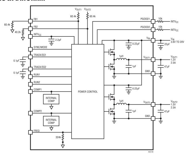
Figure 1. Simplified LTM4622 Block Diagram
