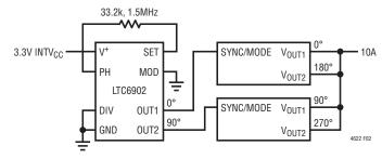
Figure 2. Example of Clock Phasing for 4-Phase Operation with LTC6902
