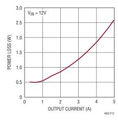
Figure 12. 5V Output Power Loss
