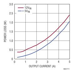
Figure 11. 3.3V Output Power Loss
