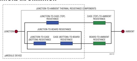
Figure 7. Graphical Representation of JESD 51-12 Thermal Coefficients
