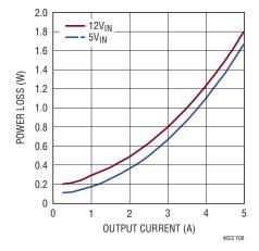
Figure 8. 1V Output Power Loss
