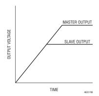
Figure 6. Output Coincident Tracking Waveform
