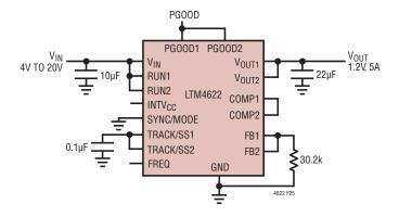
Figure 25.  $4\mbox{V}_{\mbox{\scriptsize IN}}$  to  $20\mbox{V}_{\mbox{\scriptsize IN}},$  1.2V Two Phase in Parallel 5A Design
