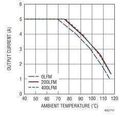
Figure 17. 5V to 2.5V Derating Curve, No Heat Sink
