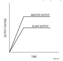
Figure 4. Output Ratiometric Tracking Waveform
