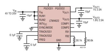
Figure 24.  $4\mbox{\ensuremath{V_{IN}}}$  to  $20\mbox{\ensuremath{V_{IN}}}, \, 1\mbox{\ensuremath{V}}$  and  $1.8\mbox{\ensuremath{V}}$  Output at  $2.5\mbox{\ensuremath{A}}$  Design
