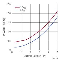
Figure 10. 2.5V Output Power Loss
