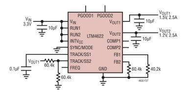
Figure 27. 3.3V<sub>IN</sub>, 1.5V and 1.2V Output at 2.5A Design with Output Coincident Tracking
