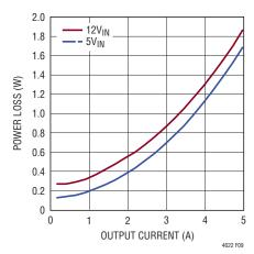
Figure 9. 1.5V Output Power Loss
