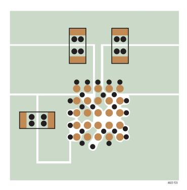
Figure 23. Recommended PCB Layout
