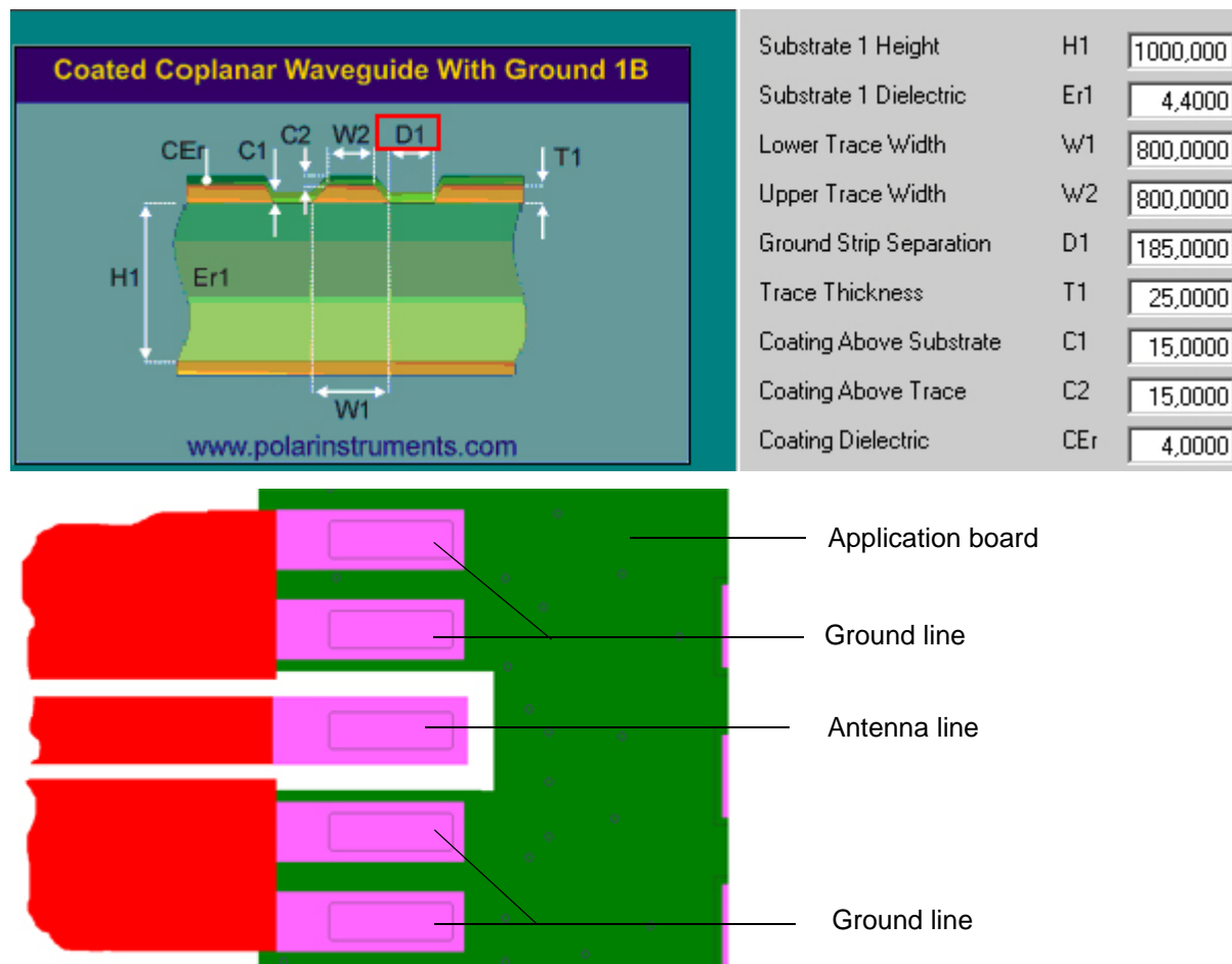
Figure 30: Micro-Stripline on 1.0mm standard FR4 2-layer PCB - example 1
