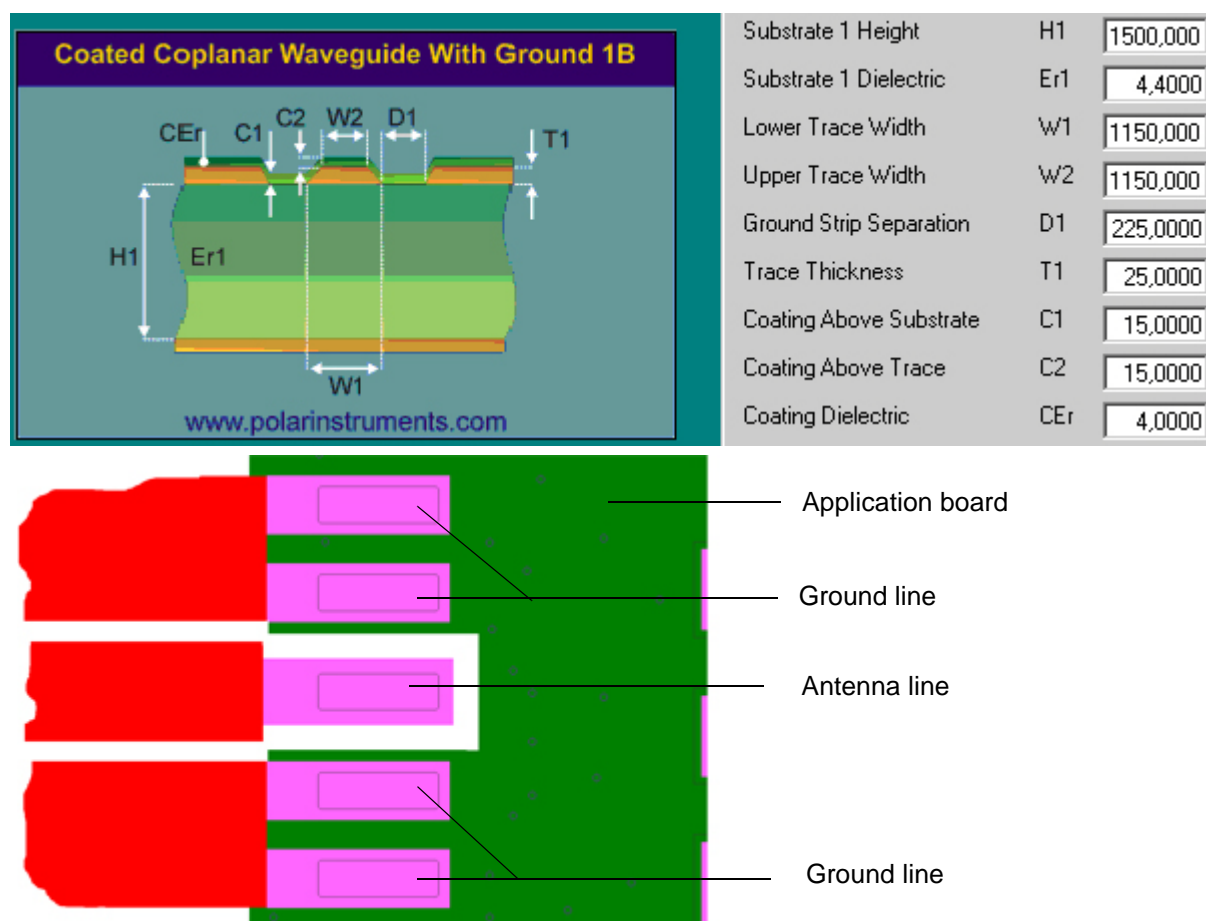
Figure 33: Micro-Stripline on 1.5mm Standard FR4 PCB - example 2
