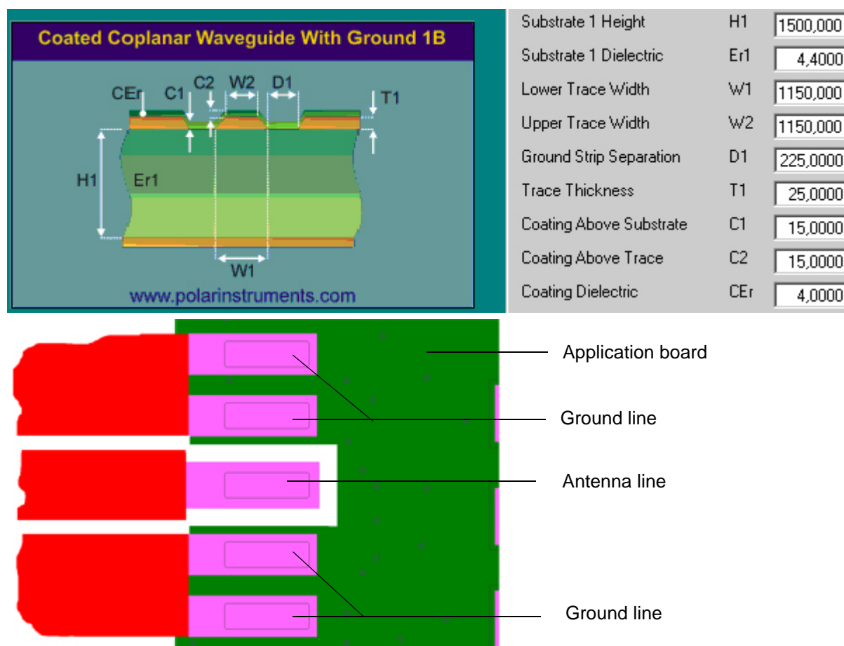
Figure 26: Micro-Stripline on 1.5mm Standard FR4 PCB - example 2
