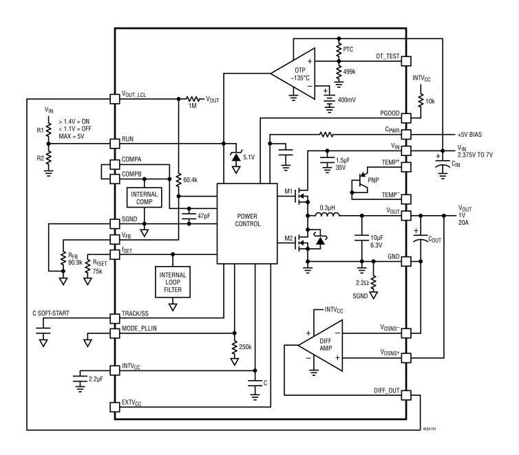
Figure 1. Simplified LTM4639 Block Diagram
