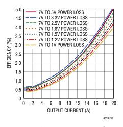
Figure 8. 3.3V Input Power Loss Curves
