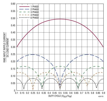
Figure 2. Normalized Input RMS Ripple Current vs Duty Cycle for One to Six µModule Regulators (Phases)
