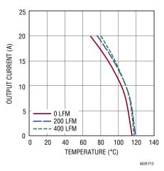
Figure 13. 7V<sub>IN</sub> to 1.0V<sub>OUT</sub> No Heat Sink
