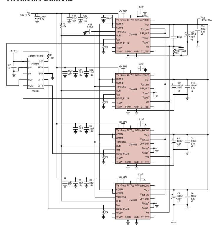
Figure 24. 1.2V, 80A, Current Sharing with 4-Phase Operation
