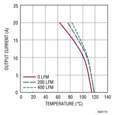
Figure 14.  $7V_{IN}$  to 1.0 $V_{OUT}$  with Heat Sink
