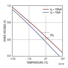
Figure 6. Diode Voltage  $V_D$  vs Temperature T(°C) for Different Bias Currents
