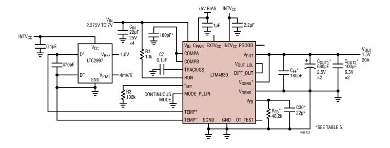
Figure 22. 2.375V to  $7\ensuremath{V_{IN}},\,1.5\ensuremath{V}$  at 20A Design
