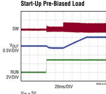
$V_{IN} = 5V$  $V_{OUT} = 1V$ ,  $V_{OUT} = 0.5V$  BIAS  $I_{OUT} = 20A$
