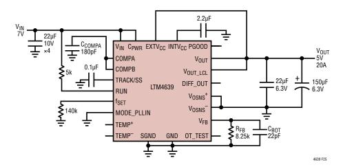
Figure 25.  $7V_{IN}$ , 5V at 20A Design
