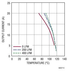
Figure 12. 5V<sub>IN</sub> to 1.0V<sub>OUT</sub> with Heat Sink
