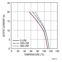
Figure 17.  $7V_{IN}$  to  $2.5V_{OUT}$  No Heat Sink
