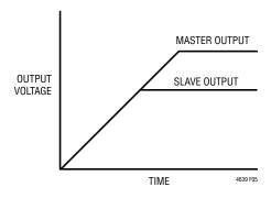
Figure 5. Output Voltage Coincident Tracking Characteristics
