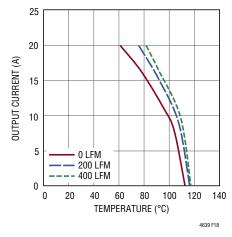
Figure 18. 7V<sub>IN</sub> to 2.5V<sub>OUT</sub> with Heat Sink
