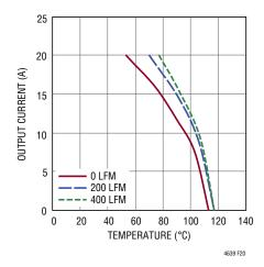
Figure 20.  $7V_{IN}$  to  $5V_{OUT}$  with Heat Sink, EXTV  $_{CC}$  = 5V,  $C_{PWR}$  = 7V
