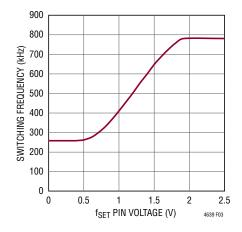
Figure 3. Relationship Between Switching Frequency and Voltage at the f<sub>SET</sub> Pin
