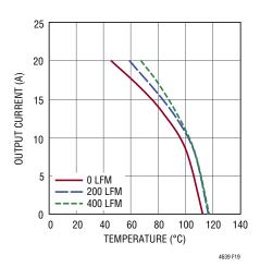
Figure 19.  $7V_{IN}$  to  $5V_{OUT}$  No Heat Sink, EXTV<sub>CC</sub> = 5V,  $C_{PWR}$  = 7V
