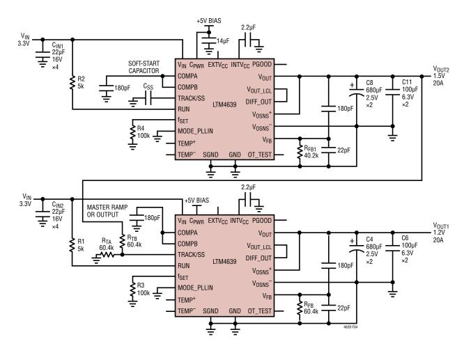
Figure 4. Dual Outputs (1.5V and 1.2V) with Tracking
