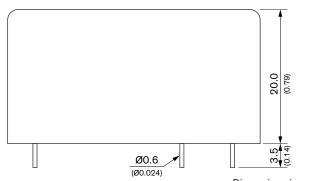
Dimensions in mm (inch) Tolerances:  $x.x \pm 0.5 (\pm 0.02)$
