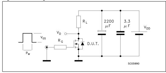
1. Max driver  $V_{GS}$  slope = 1V/ns (no DUT)
