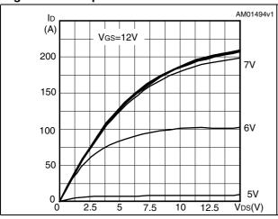
Figure 7. Transfer characteristics
